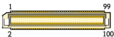
Figure 45: ETX connector X1, X2, X3 and X4 diagram
