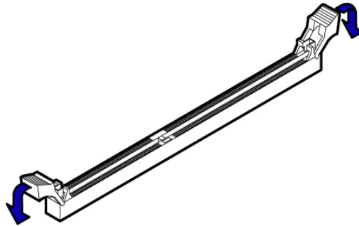
Figure 39: Unlocking the memory DIMM slot
